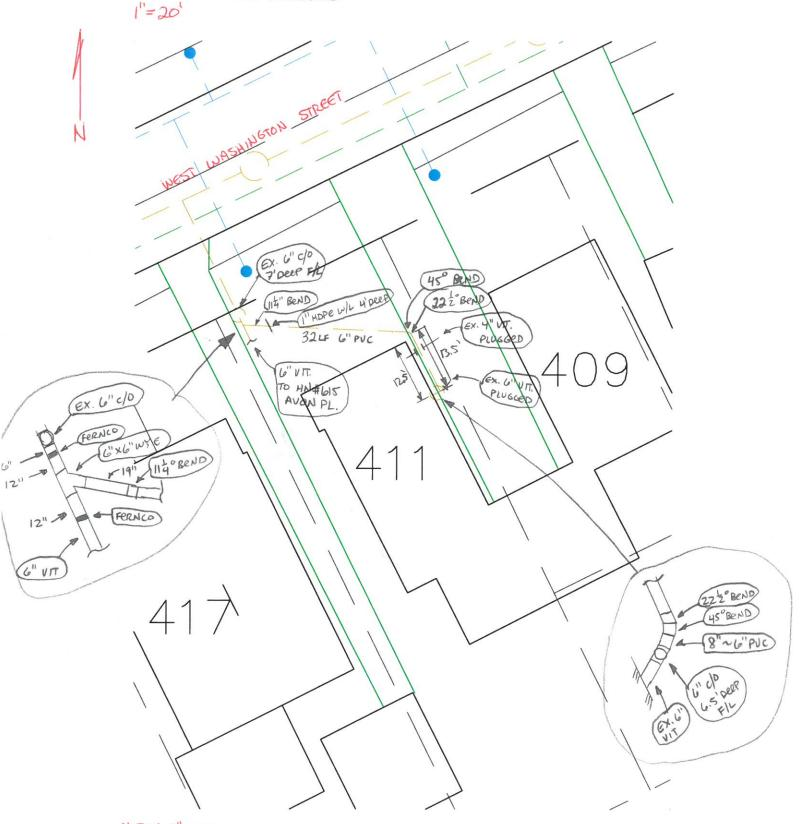
NOTE: I" HOPE WATER SERVICE TO HN # 411 WAS CUT AND REATTACHED WITH 2 1" COMP. COUPLINGS 4' DEEP AND 4' NE OF DRIVEWAY.
